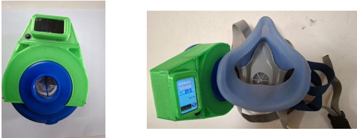
Figure 6: General view of the real-time pressure drop monitoring unit on respirator filters with display
